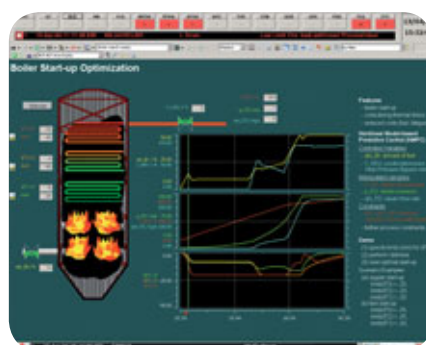
Typical operating screen for optimizing boiler startup
