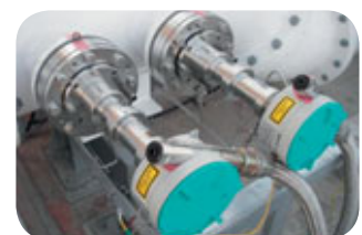
Redundant in-situ oxygen measurement with laser analyzers
