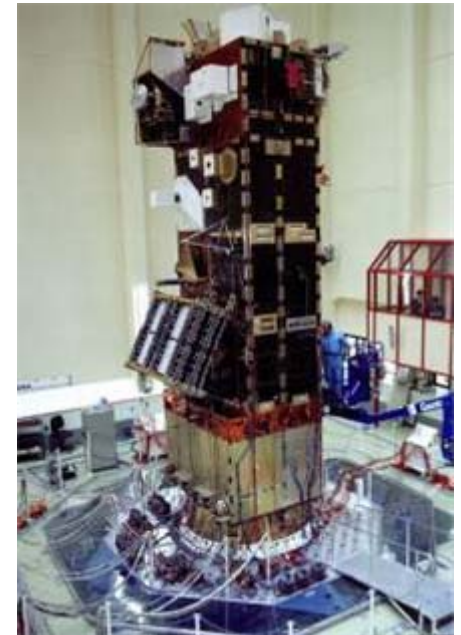
ENVISAT structural model for qualification in vibration
