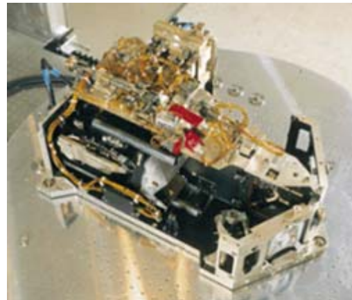
ENVISAT structural model for qualification in vibration
