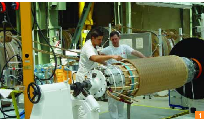
1 Transformer coil winding in an ABB factory.
