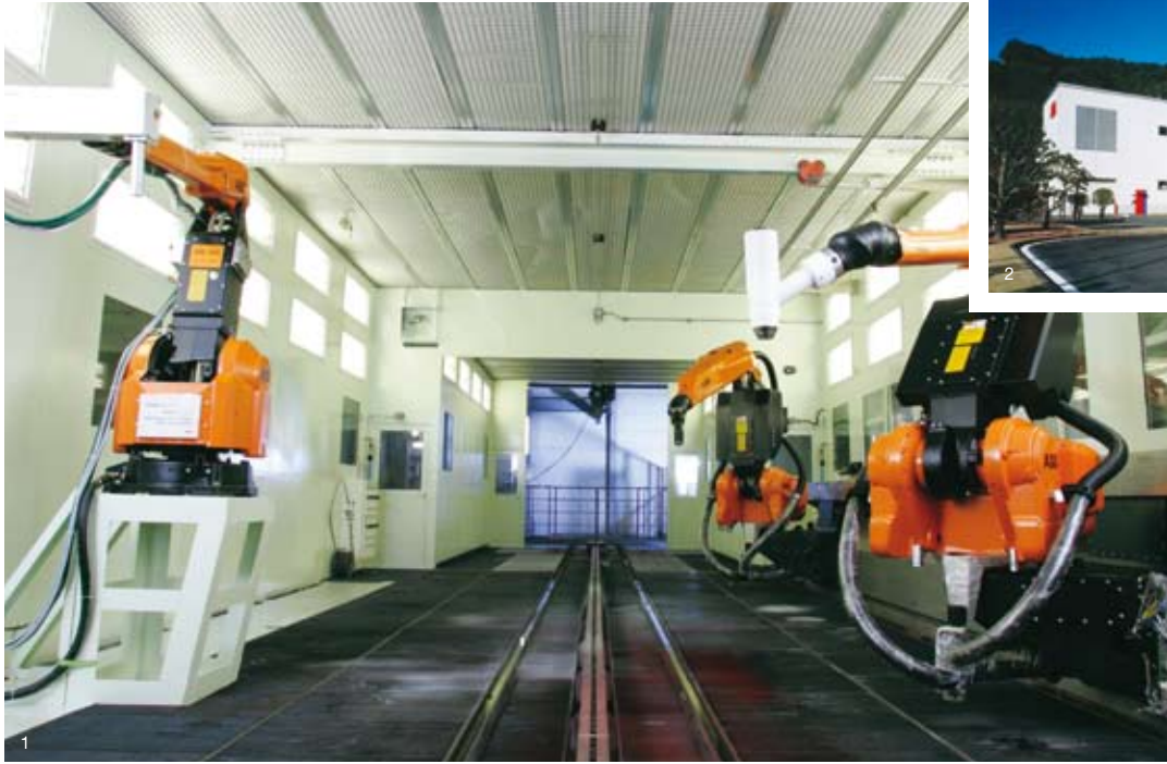
1 Test paint booth in the Technical Center, equipped with state-of-the-art paint robots. 2 The ABB Japan Technical Center in Shizuoka Prefecture.
