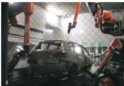
5 ABB's Module System allows for shorter paint booths and reduced energy costs. 6 The revolutionary 3 Wet System combines three formerly separate paint operations for reduction of VOC emissions and energy costs.
