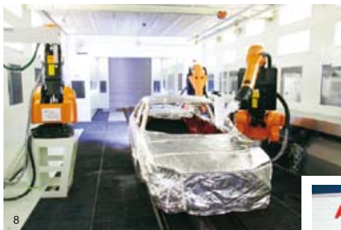
8 Paint booth for testing, equipped with state-of-the-art paint robots
