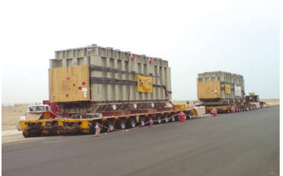
Large power transformers en route to Sulaibiyah, Fintas and Jabriya in Kuwait.
